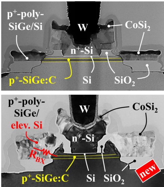
Fig. 2: TEM cross-sections of the old (top) and new SiGe HBTs (bottom). The major change is the elevated external base leading to a reduction of the external base resistance ( $R_{BX}$ ), being beneficial to  $f_{max}$ .
