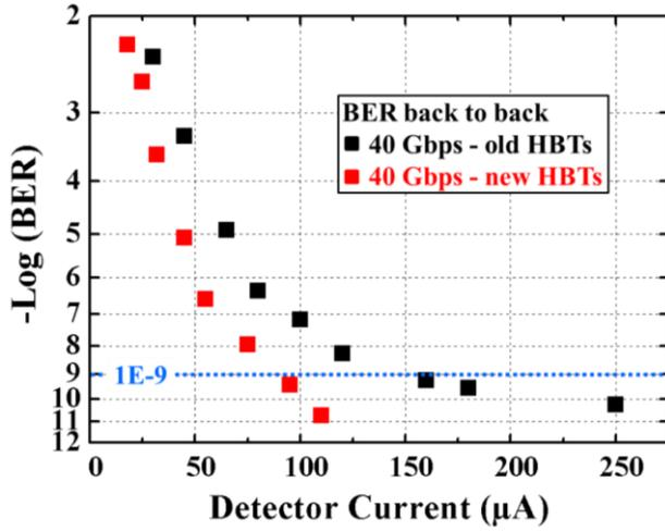
Fig. 6: BER vs. PD current for 40 Gbps: Comparison of monolithically integrated receivers with new and old HBTs.
