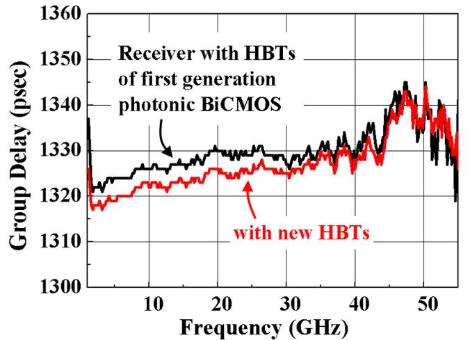
Fig. 4: Group delay vs. frequency of monolithically integrated photonic receivers with same design, fabricated in IHP's first generation photonic BiCMOS process or in an advanced process version featuring faster SiGe HBTs.
