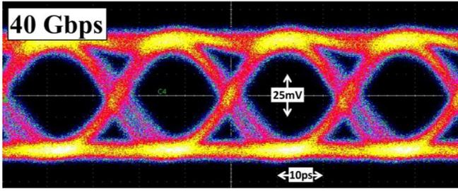
Fig. 5: Eye-diagram at 40 Gbps ( $2^{31}$ -1 PRBS) of a monolithically integrated direct receiver fabricated in the advanced photonic BiCMOS process. PD current: 260  $\mu$ A.
