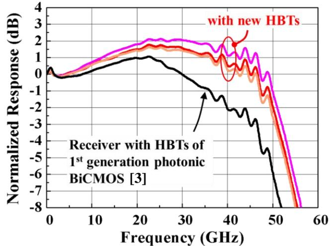
Fig. 3: Normalized O-E frequency response of monolithically integrated photonic direct receivers with identical design, fabricated in IHP's first generation photonic BiCMOS process or in an advanced process version featuring faster SiGe HBTs (three chips of one wafer were measured for this case). Measurements were carried out at  $\lambda = 1.55 \mu\text{m}$ .
