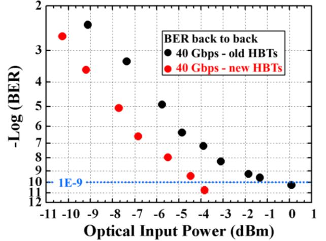
Fig. 7: BER vs. optical input power for 40 Gbps: Comparison of monolithically integrated receivers with new and old HBTs.
